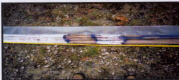
TCE stains from fractures in a 3 in. core hole (note the boot toes for scale)
