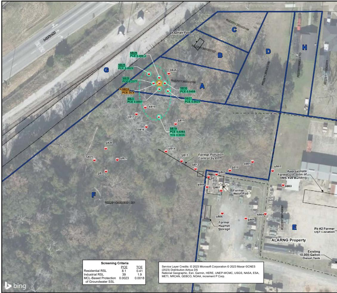
Figure 1-8 Brookley Lower S ubsurface Soil Sample Results for TCE and
